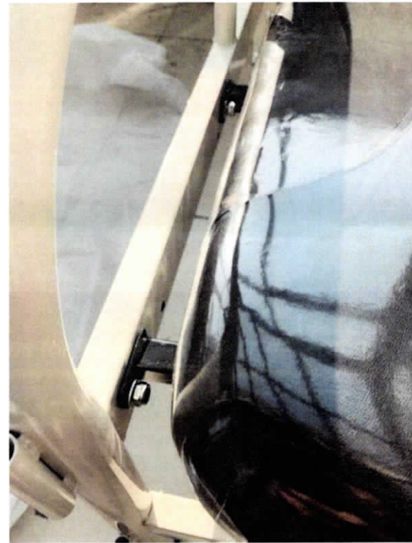
3-4: Fix the seat to the legs with the bolts & nuts.
