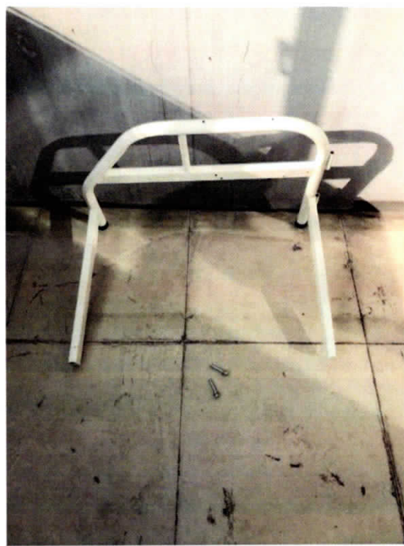
1-4: Using the bolts to connect the leg to the beam.
