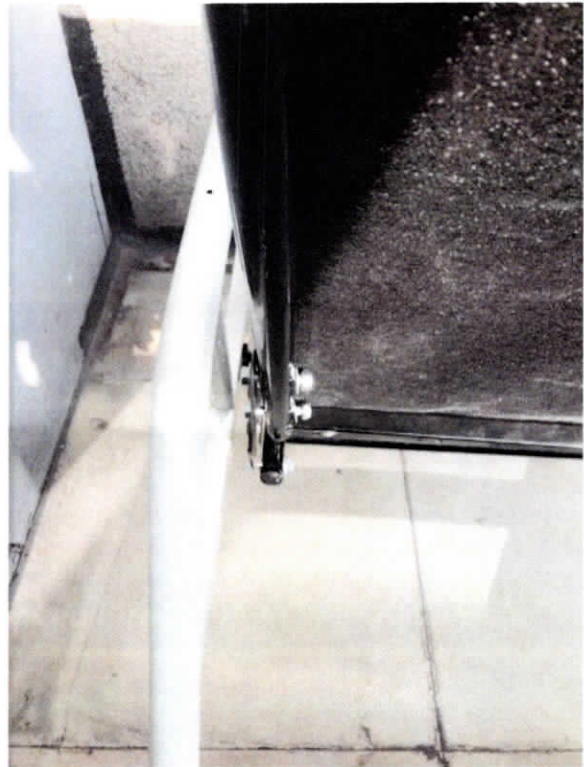
4-4: Connect the backrest to the "L" shape with bolts & nuts.
