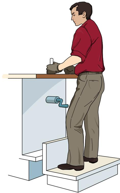
Figure 30-6 Height-adjustable work stations
